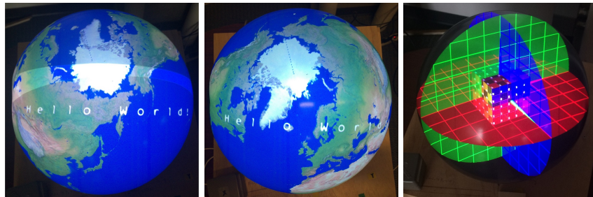
Fig. 8. View-independent application (a) after geometry calibration (b) after blending (c) View-dependent application.
